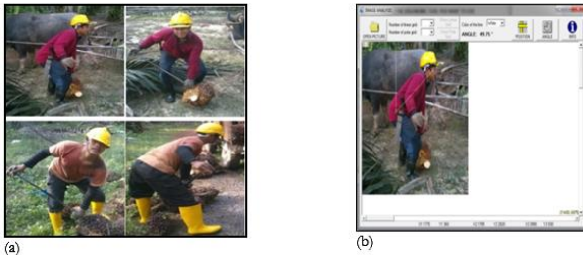
Fig. 5: (a) Various angles of task loading FFBs into lorry; (b) Hip posture angle
