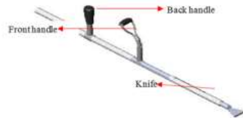
Fig. 6: New design harvesting tool.
