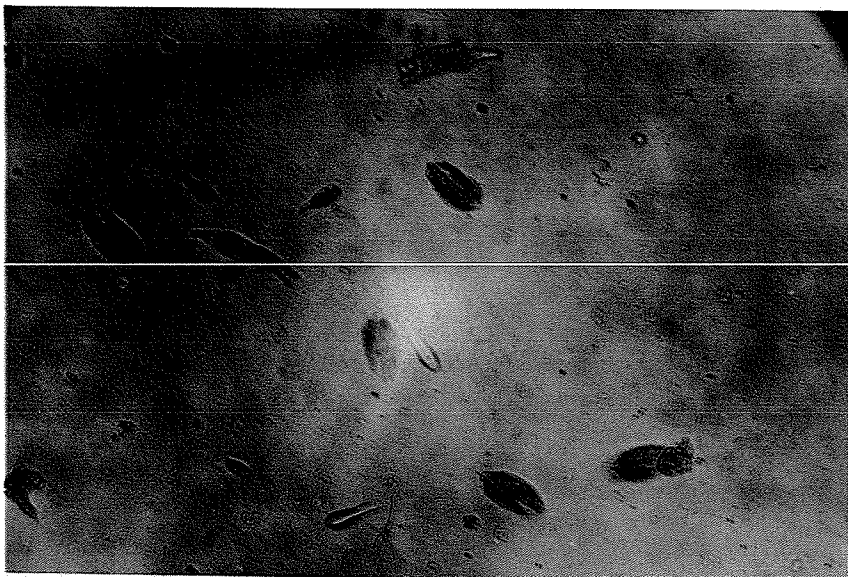
Photomicrograph of Free Swimming Protozoa and Rotifers Typical for the Aerobic Plastic Media Unit
