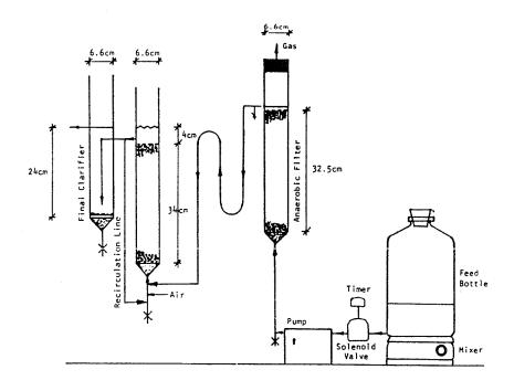
Fig.1: Schematic Diagram of two Stage System.
