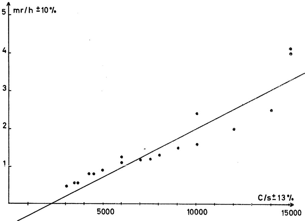
Fig. 2: Comparison between counts per second and millirontgens per hour for environmental radioactivity.
