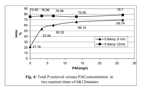
In reaction time of 6 min,  $27 \text{ mgL}^{-1}$  PAC additions, can improve the efficiency of P-removal up to 50%, but similar improvement cannot be gained in 12min. Tables 4-5 show the concentrations of T.P after electrochemical process on different alum and ferrous sulfate
