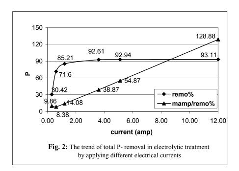
**Fig. 2:** shows the percentages of P- removal versus electrical current in 10 min reaction time. As it is shown, removal efficiency for phosphorous can be improved by increasing electrical current. The minimum ratio of current to 1% P- removal could be gained by imposing 0.6 amp current.
