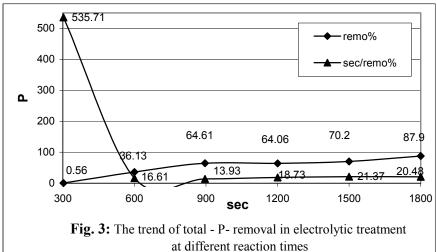
The changes in total P- removal efficiency versus reaction time can be seen in figure 3.
