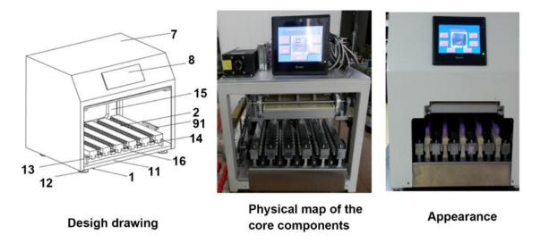
**Fig. 1 A:** new type of blood vacuum cap opening and closing machine. Note 1. Mounting base; 11. Fixing and supporting transverse plate; 12. Leg of the mounting base; 13. Left supporting vertical plate; 14. Right supporting vertical plate; 15. Fixing and supporting vertical plate; 16. Transverse guide rail; 2. Gripping mechanism; 7. Sheet metal shell; 8. Touchscreen; 91. Photoelectric sensor
