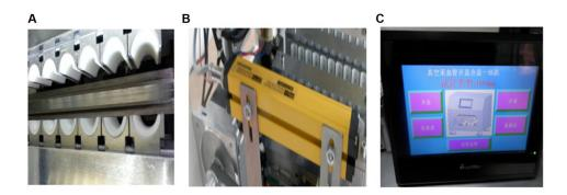
Fig. 2: Physical map of core components. A: Gripping head. B: Alarm device. C: Touchsreen
