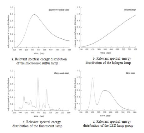
Fig. 2: Relevant spectral energy distributions of four artificial light sources
